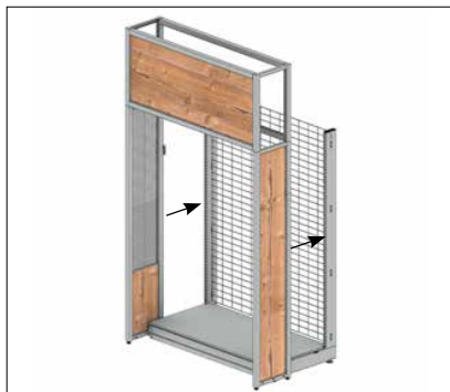
Mounting the gondola head superstructure with advertising frame
